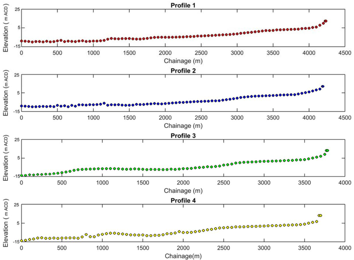
*Figure 21: Beach profiles used as an input for extreme event simulations, profiles include height of any parapets present*
