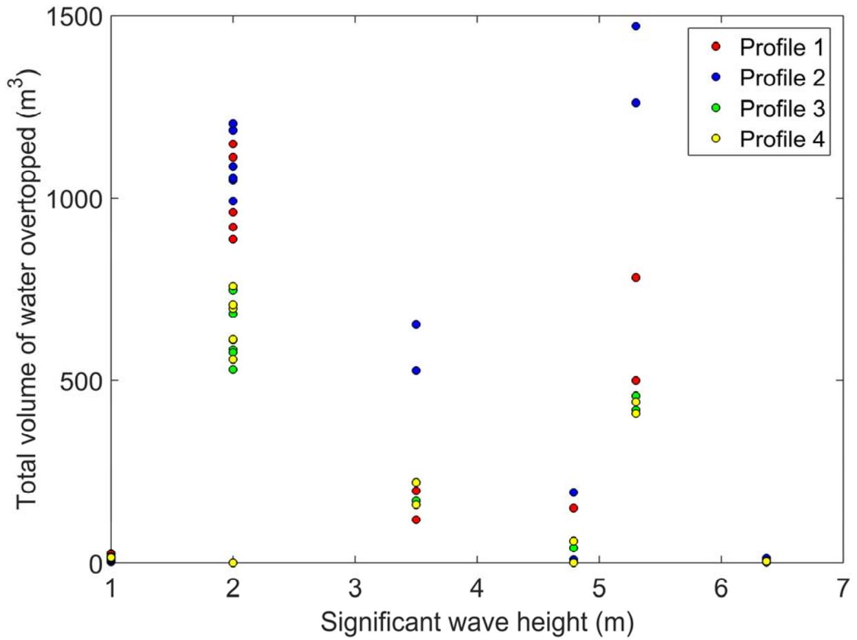
*Figure 30: Mean total overtopping volume for each profile for a selection of scenarios simulated.*
