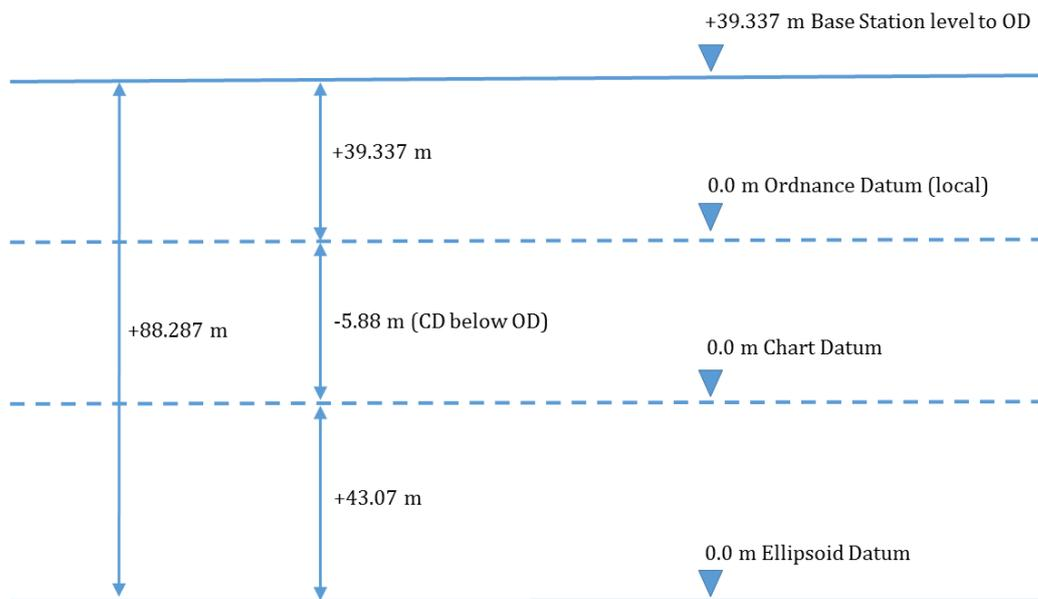
**Figure A1: Ellipsoid Datum, Ordnance Datum (local) and Chart Datum relationship for Jersey, offsets provided by GeoSurf survey in 2012.**
